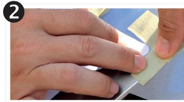
Measure end position before applying glue and mark with easily removable adhesive tape (e.g. paint masking tape).
