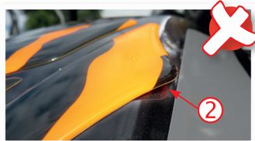
② Attempting to apply the adhesive to beading will cause the material to be under too much tension and **will come loose after a short time**.
