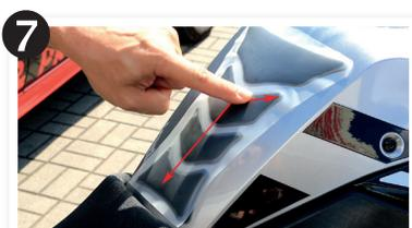
It is recommended to apply the pad from the center outwards. **Do not apply too much pressure in order to avoid unnecessary „shifting“ of the material.** Instead, apply with normal, controlled force.
