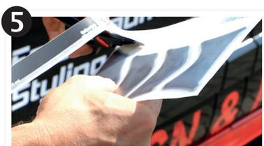
Cut the shape roughly to size. (For products with transfer tape - do not cut away too much!)
