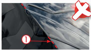
① **Do not apply the adhesive over beading, edges and bends that are too sharp**, otherwise the adhesive surface cannot
